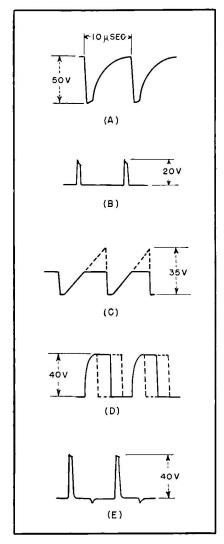
FIG. 2-Waveforms, oscillator to output
