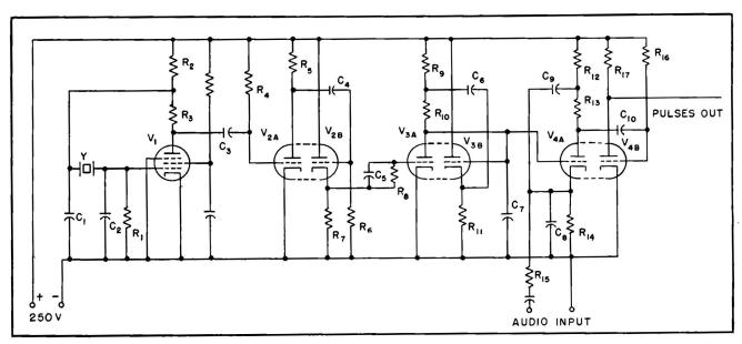
FIG. 1—The modulator proper showing the crystal oscillator, clipper, sawtooth generator and bootstrap cathode follower, and f-m pulse output tubes. The frequency multiplier stages that follow are conventional
